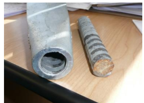
Stripped threads - screw in connection detail
