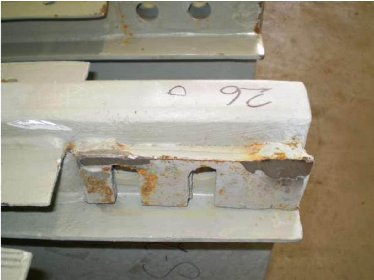
**Figure 1: Poorly fabricated steelwork – Glass barrier bridge truss (Australian project)**
