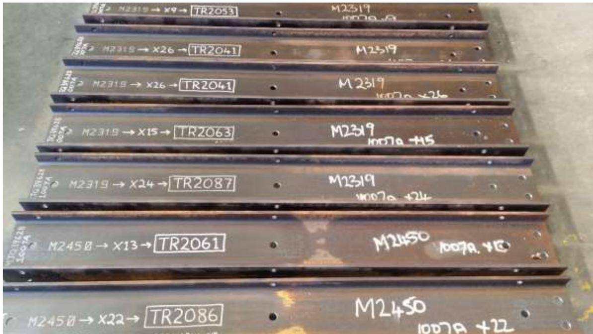
**Figure 2: An example of component marking in the fabricator's workshop**
