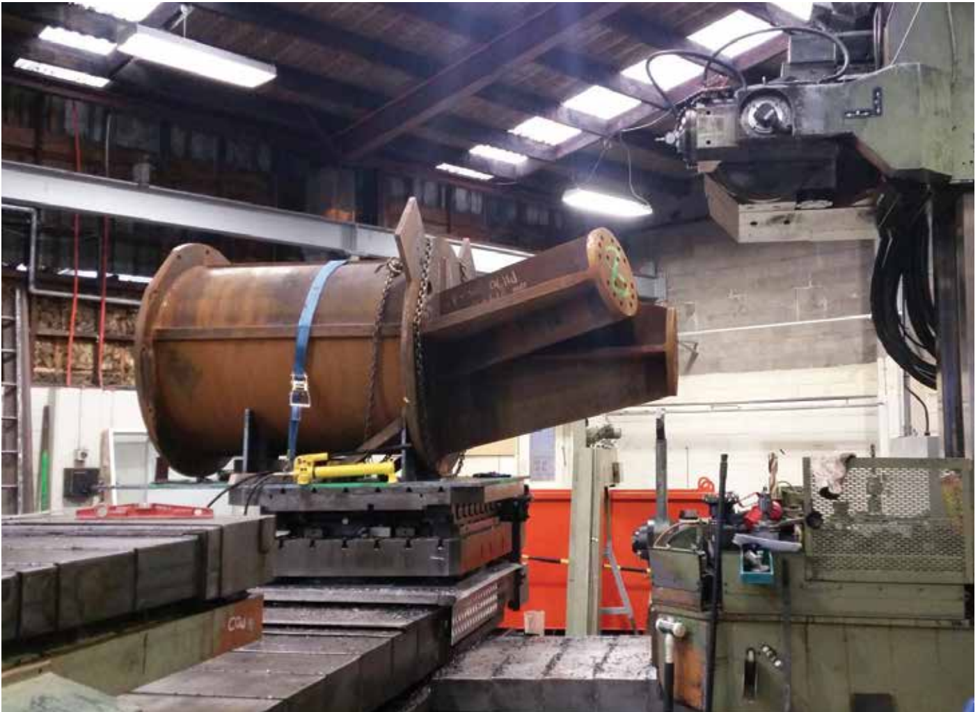
Large five-tonne, ground-level fabricated node section on machine table, about to have diagrid face plates machined.
