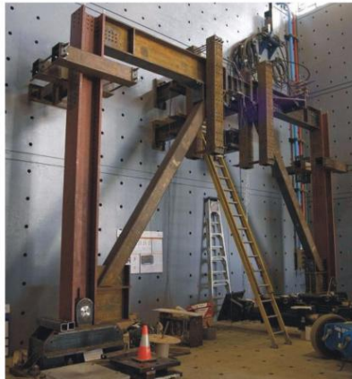
Figure 6: EBF frame and test setup (Mansour, 2010)
