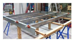
(a) LSB studs and Channel section tracks
