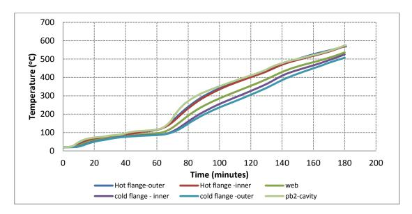
Figure 8. Time-Temperature profiles of the steel stud surfaces with time in Test 1
