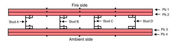
Figure 4. Locations of thermocouples
