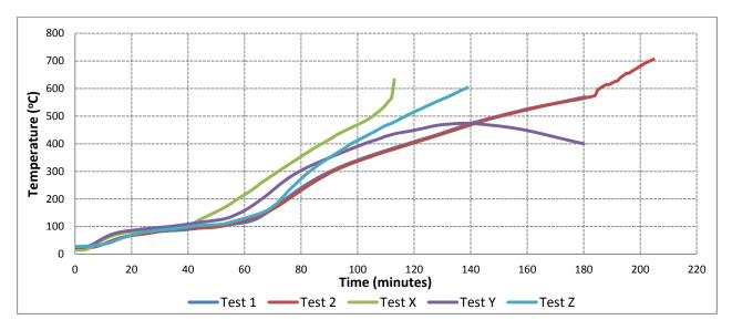
Figure 12. Hot flange temperature of failed studs
