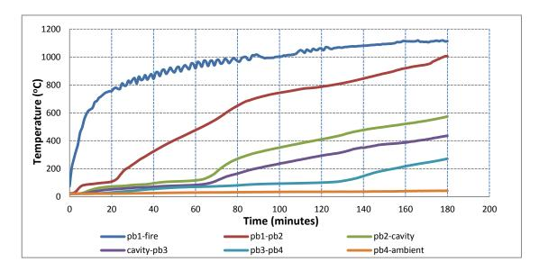
Figure 7. Time-Temperature profiles of the plasterboard surfaces in Test 1
