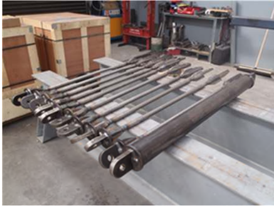
Figure 9: Mild steel fuse rods under fabrication and prior to being encased and grouted
