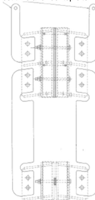
**Figure 11 – FEGL Shop Drawing of Clamp Installation Jigs**
