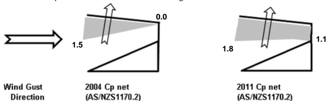
**Figure 5 – Cantilever Roof Wind Pressure Coefficients in 1170.2**
