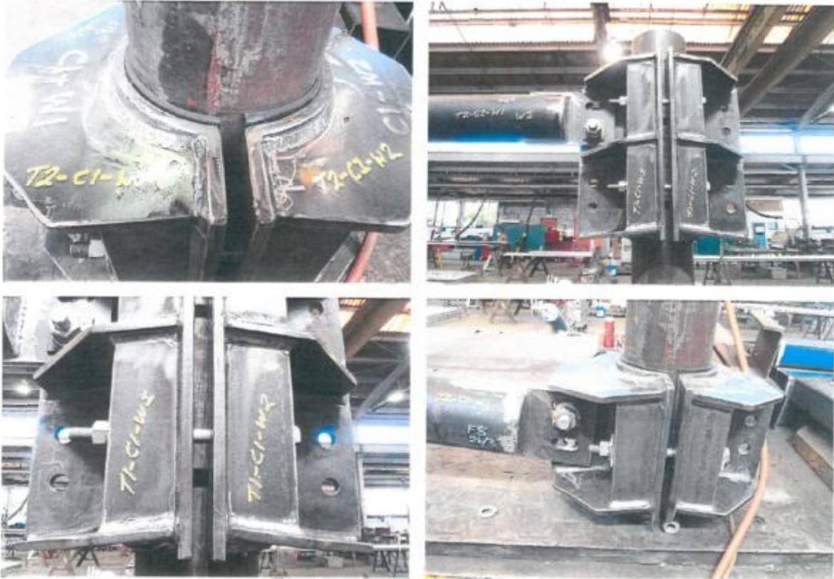
Figure 12 – Photos from FEGL’s workshop depicting the mock assembly of components
