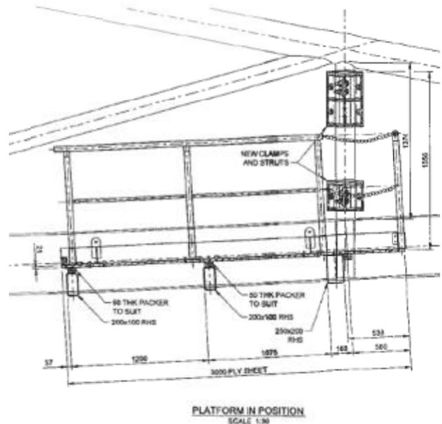
Figure 10 – FEGL Shop Drawing of Craned Access Platforms
