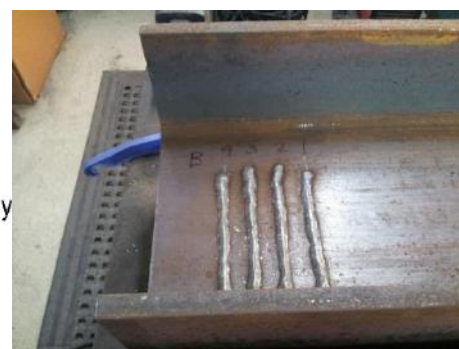
Figure 2 A universal column showing deposited weld metal as used for the CVN tests
