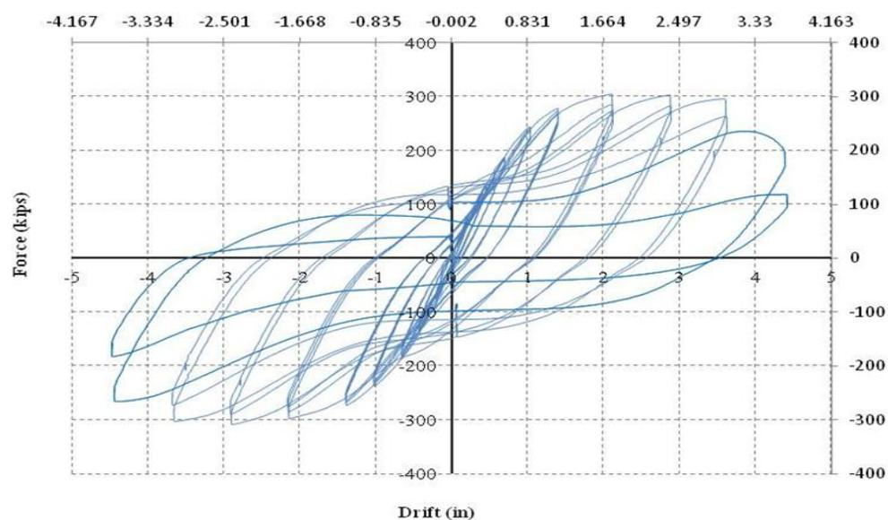
Figure 6: hysteretic force-displacement curve for Specimen CFSSP-NB1
