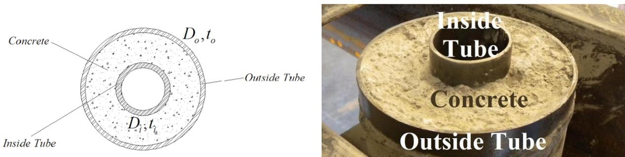
Figure 7. Concrete Filled Double Skin Tube
