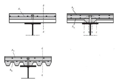
Figure 4: Typical potential surfaces of shear failure where decking is used. (Hicks, 2011)
