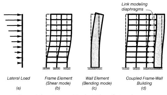
Figure 1. Deformation compatibility of a dual frame. (Bull, 2004)
