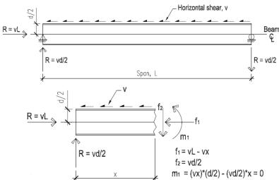
Figure 10. Consideration of any secondary moments for a simple supported collector beam (Burmeister, 2008).
