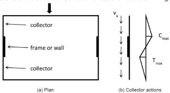
Figure 3. Diaphragm Collectors. (Sabelli et al. 2011)
