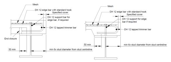
Figure 6: Spandrel beam reinforcement. (Clifton, El Sarraf, 2005)
