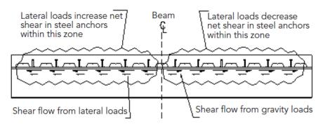
Figure 9: Shear flow due to Gravity and Lateral Loads in Combination. (Burmeister, 2008).
