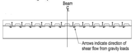
Figure 8: Shear Flow due to Gravity Loads Only (Burmeister, 2008).
