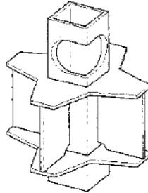
**Figure 6: Two-way Moment Frame - External Diaphragm**
