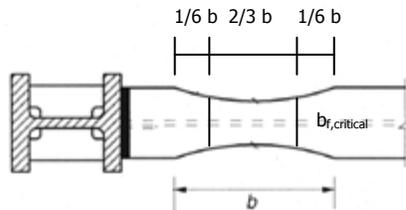
**Figure 5: Critical Section Location for Flange Slenderness Check**
