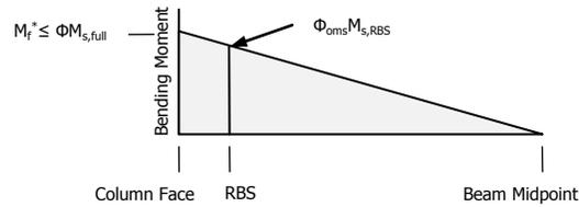
**Figure 2: Column Face Bending Moment**
