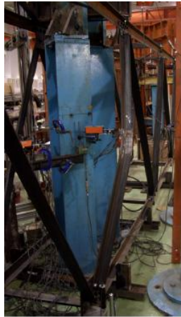
Figure 19 Weak axis buckling mode (Chan and Cho, 2008)
